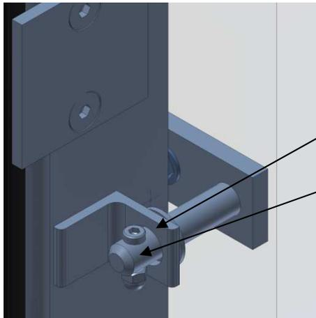
Fig. 2.3.3.1 Lock with screw, factory design
