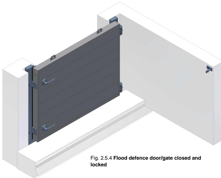
**Fig. 2.5.4 Flood defence door/gate closed and locked**
