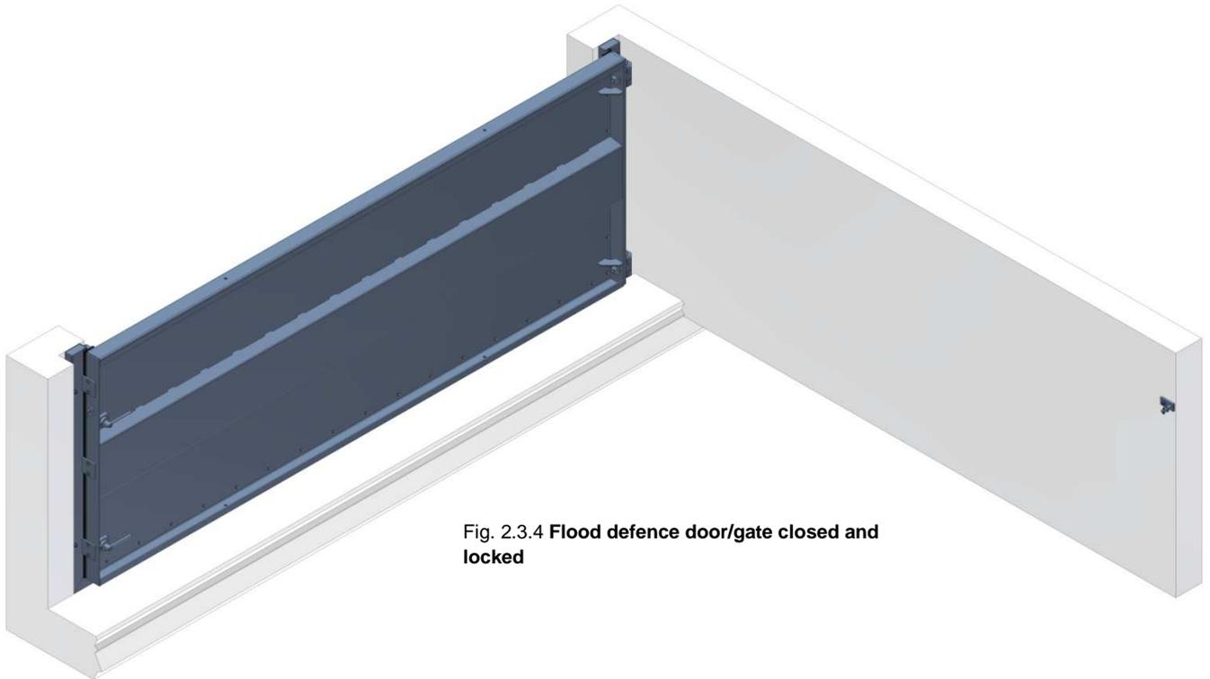
**Fig. 2.3.4 Flood defence door/gate closed and locked**
