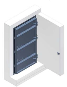
Fig. 1.4.4 Flood defence door/gate closed and locked
