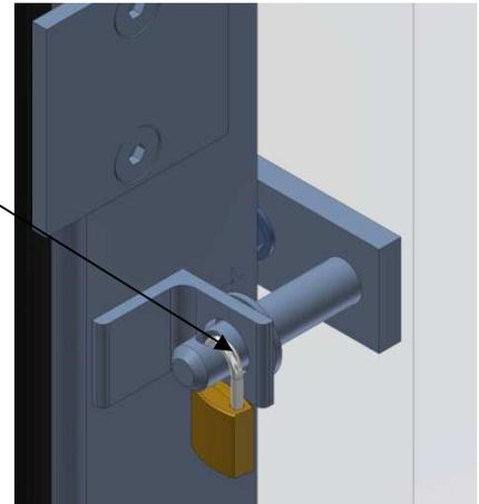
Fig. 2.3.3.2 Lock, optionally with padlock
