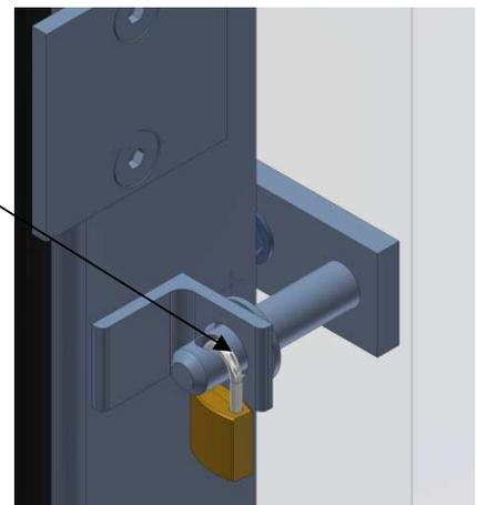
Fig. 1.4.3.2 Lock, optionally with padlock
