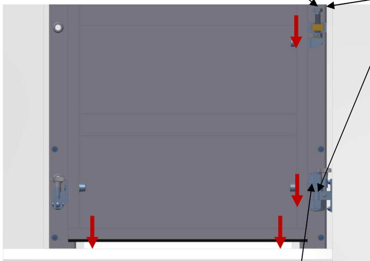
Fig. 1.2.3.6 Lowering the door Position A
