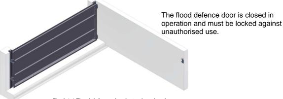
Fig. 2.1.4 Flood defence door/gate closed and locked
