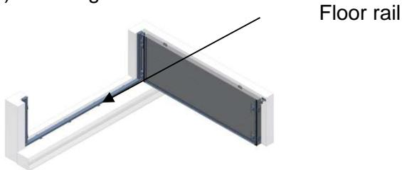
Fig. 2.6.3.3 Cleaning the floor rail
