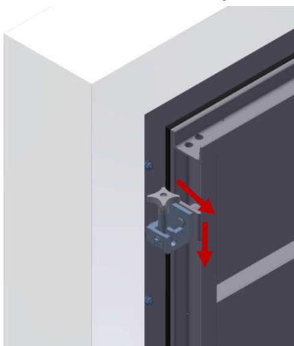
To close the door, bring the two closure mechanisms into horizontal position
