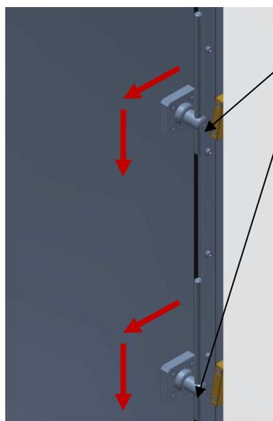
To lock the gate, bring the two closure mechanisms into horizontal position.
