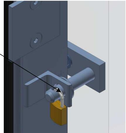
Fig. 2.4.3.2 Lock, optionally with padlock
