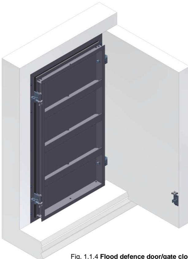
Fig. 1.1.4 Flood defence door/gate closed and
