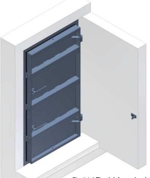
Fig. 1.1.4 Flood defence door/gate closed and locked
