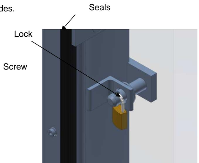
Fig. 1.3.3.2 Lock, optionally with padlock
