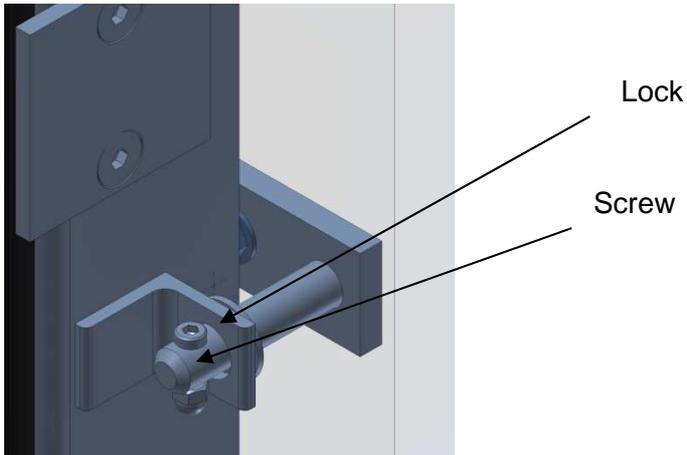
Fig. 2.4.3.1 Lock with screw factory design
