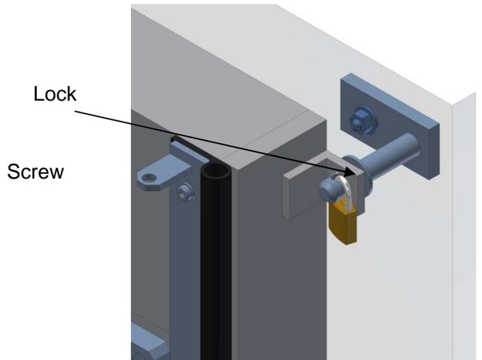
Fig. 2.6.3.2 Locking, optionally with padlock
