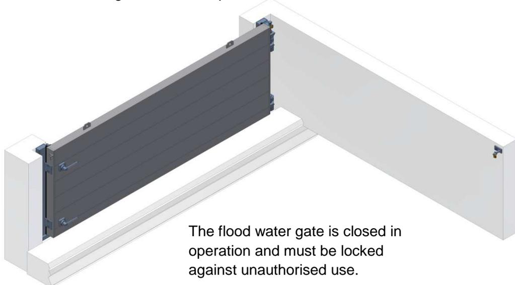
Fig. 2.6.4 Flood defence door/gate closed and locked
