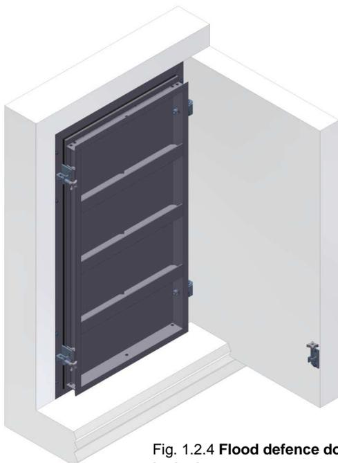
Fig. 1.2.4 Flood defence door/gate closed and locked
